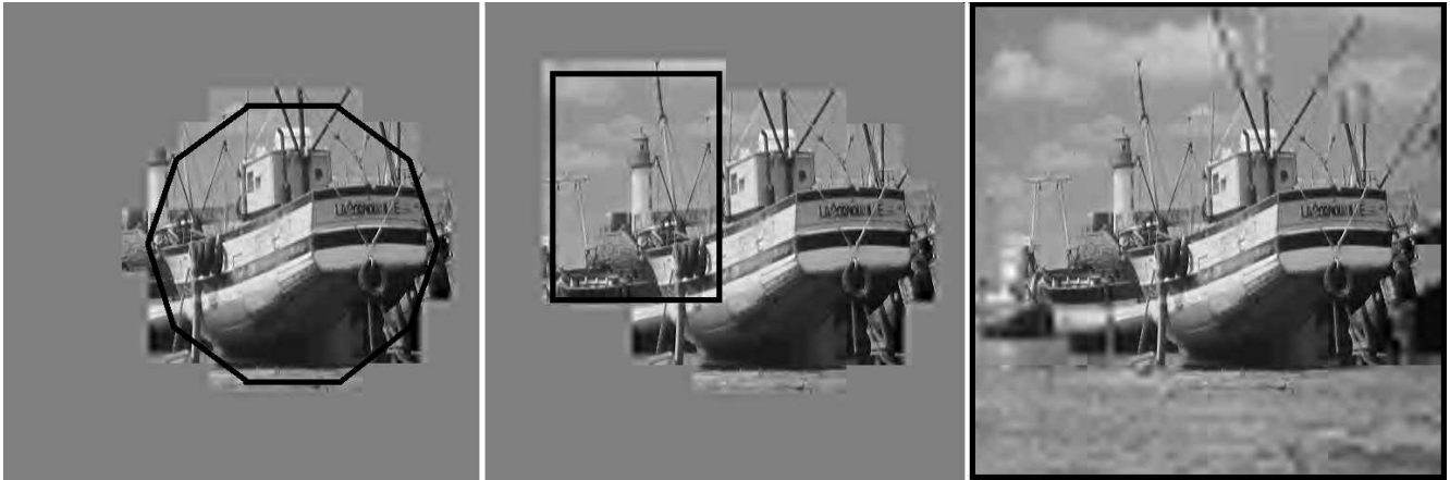
Fig. 3. Dynamic Regions of Interest with JPEG2000 using the proposed method (image after 9 (left), 12 (center) and 15 (right) seconds using a GSM connection).
